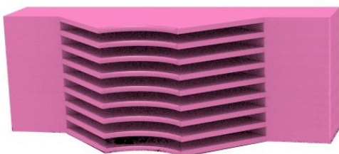
Figure 3: The thin slices of the gaseous volume passes between the conducting fins of a hot block where they heat up quickly.
