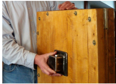
Picture 4: Sealing cap covering vital parts of the "Revolving Dynamic Link" control system.
