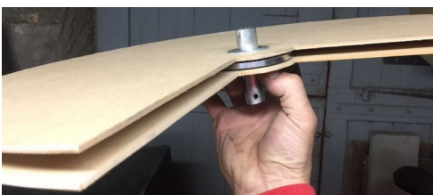
Picture 1: A two-layer revolving shutter RS with cut out quarter openings to carry the work generating volume
