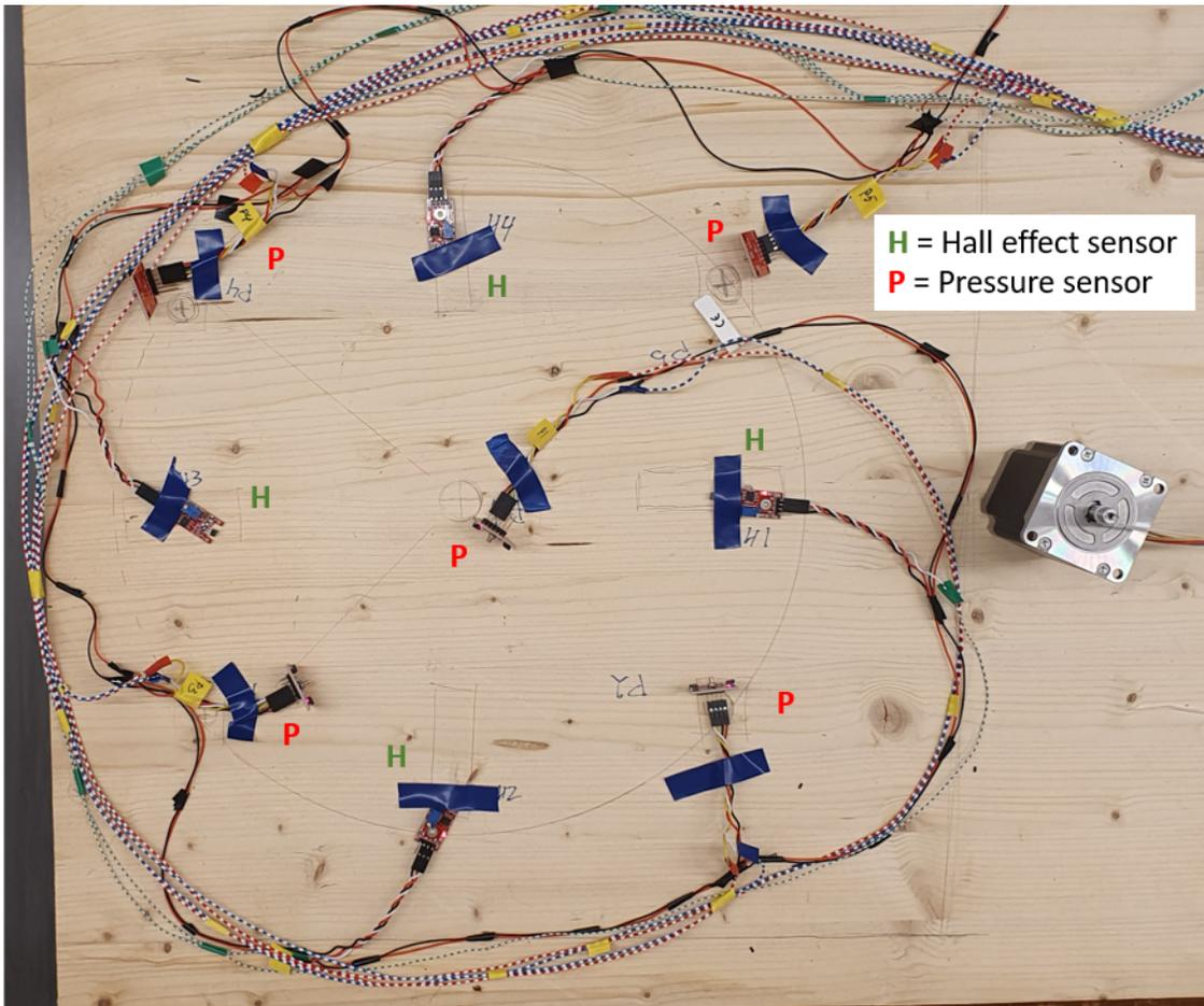
Figure 13: A test assembly of the approximate placement of the sensors in the GREC. A drawn RS is shown on a wooden plate to illustrate where the sensors are placed.
