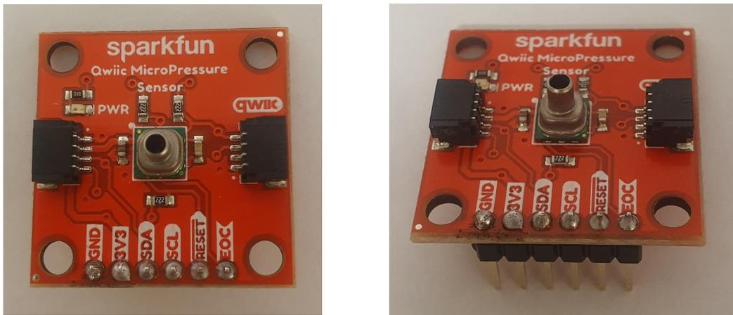
Figure 6: The micropressure sparkfun sensor.
