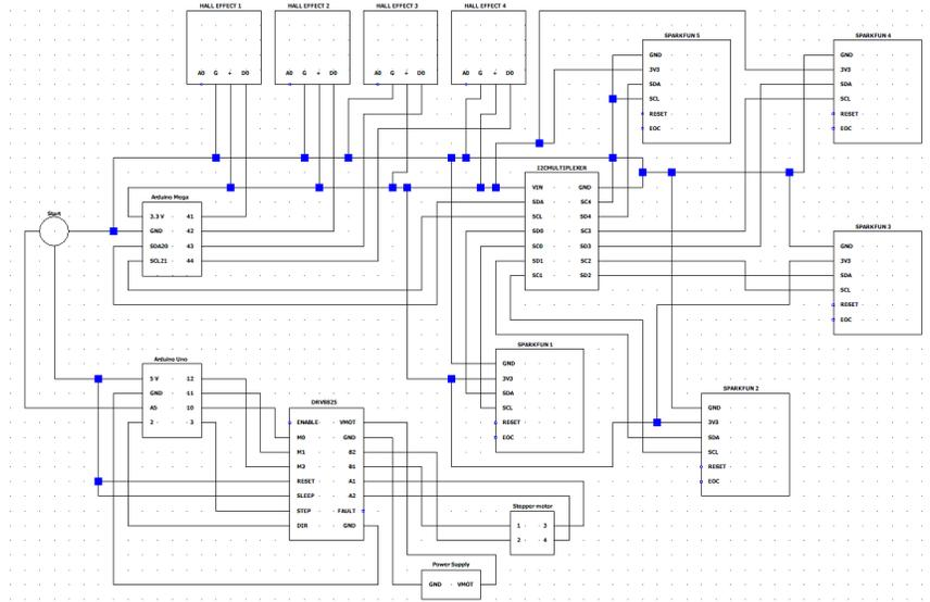
Figure 12: Figure showing the wiring diagram designed of the components for the GREC. For a clearer picture, see Appendix B
