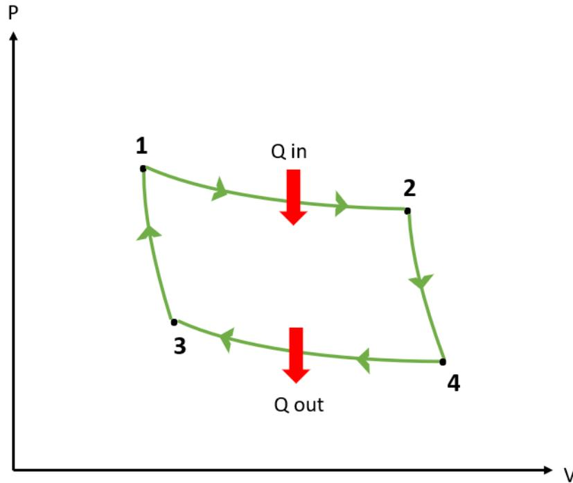
Figure 1: Pressure-Volume diagram illustrating the Carnot cycle. Red arrow  $Q_{in}$  illustrates heat source that adds energy, whereas  $Q_{out}$  illustrates the cold source where energy is reduced.
