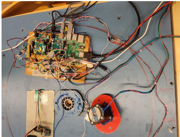
Figure 3: A picture of the current electric system for the GREC. A stepper-motor glued to a red plate is visible in the picture as well as the Arduinos and the Raspberry Pi
