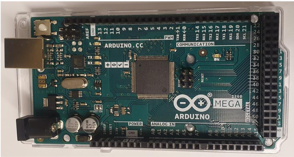
Figure 4: A picture taken with cellphone camera showing the Arduino Mega 2560 used for the project.
