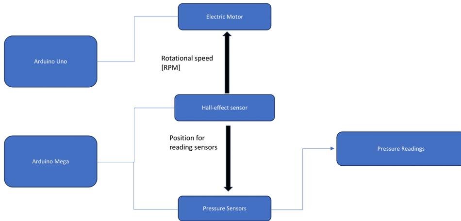
Figure 11: A schematic picture over the structure for the code controlling the system. This is implemented using Arduino IDE and the complete code can be found in Appendix A.
