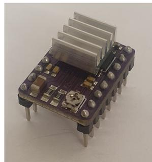
Figure 10: The stepper motor driver DRV8825.
