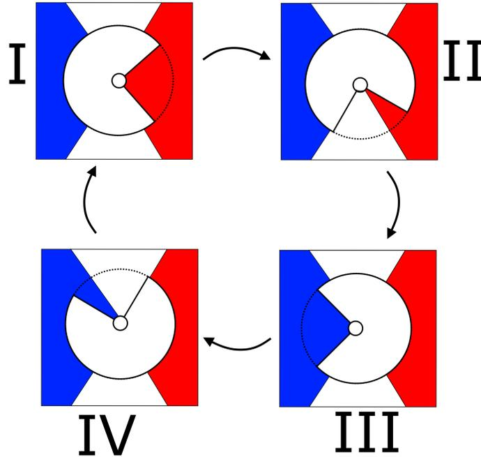
Figure 2: Illustration of a cycle of the GREC. Red part illustrates the heat source, and the blue part the cold source.
