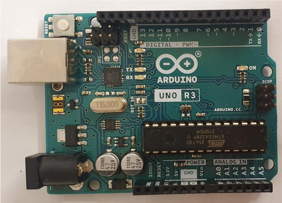
Figure 5: A picture taken with cellphone camera showing the Arduino Uno used for the project.
