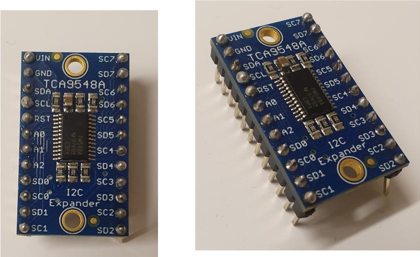
Figure 7: The I2C Multiplexer component.
